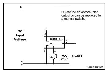
Figure 22. Active-on (Fail Safe) Remove ON/OFF.
