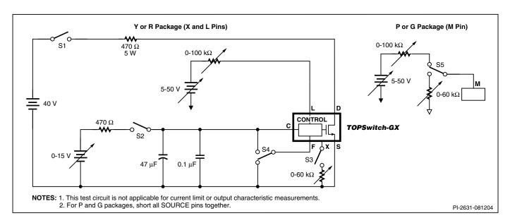
Figure 53. TOPSwitch-GX General Test Circuit.
