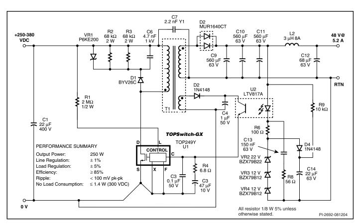
Figure 43. 250 W, 48 V Power Supply using TOP249.
