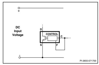
Figure 13. Full Frequency Operation (132 kHz).
