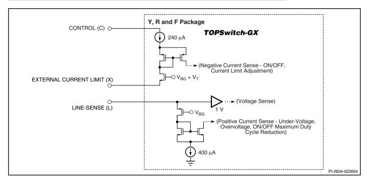
Figure 12a. LINE-SENSE (L), and EXTERNAL CURRENT LIMIT (X) Pin Input Simplified Schematic.
