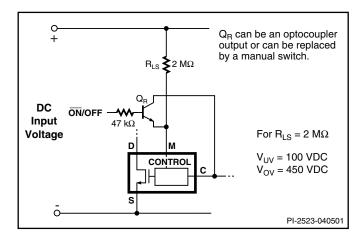
Figure 40. Active-off Remote ON/OFF with LINE-SENSE.
