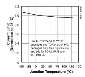
Figure 60. External Current Limit vs. Temperature with  $R_{II} = 12 \text{ k}\Omega$ .
