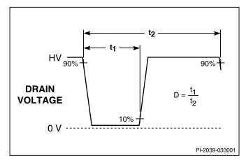
Figure 50. Duty Cycle Measurement.
