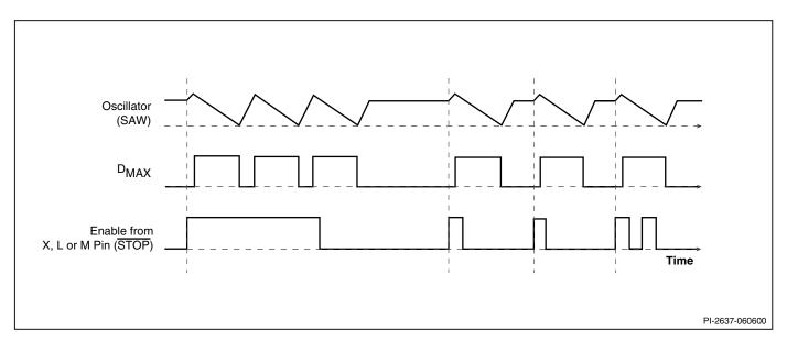
Figure 10. Synchronization Timing Diagram.
