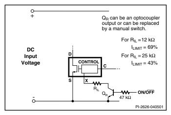
Figure 24. Active-on Remote ON/OFF with Externally Set Current
