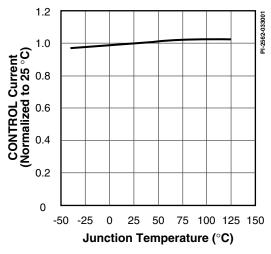
Figure 65. Control Current Out at 0% Duty Cycle vs. Temperaure.
