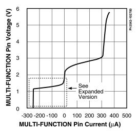
Figure 64a. MULTI-FUNCTION Pin Voltage vs. Current.
