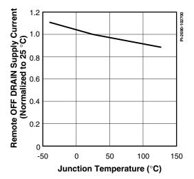
Figure 71. Remote OFF DRAIN Supply Current vs. Temperature.
