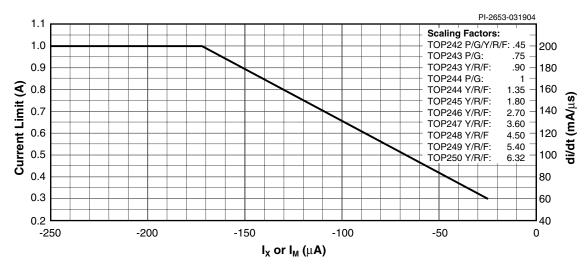
Figure 54a. Current Limit vs. X or M Pin Current (see Figures 55a and 56a for TOP245P/G and TOP246P/G).
