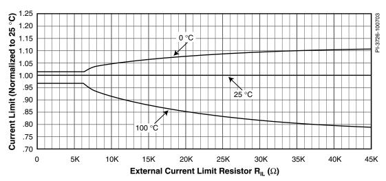
Figure 56c. External Current Limit vs. External Current Limit Resistance at 0 °C, 25 °C and 100 °C Junction Temperature (TOP246P/G only).
