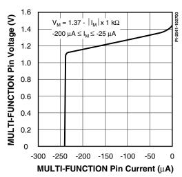
Figure 64b. MULTI-FUNCTION Pin Voltage vs. Current (Expanded).
