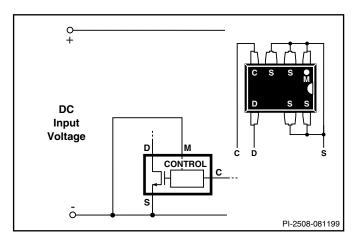
Figure 30. Three Terminal Operation (MULIT-FUNCTION Features Disabled).
