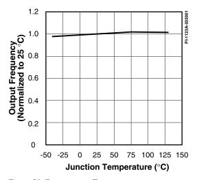
Figure 58. Frequency vs. Temperature.
