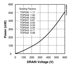
Figure 70. DRAIN Capacitance Power.
