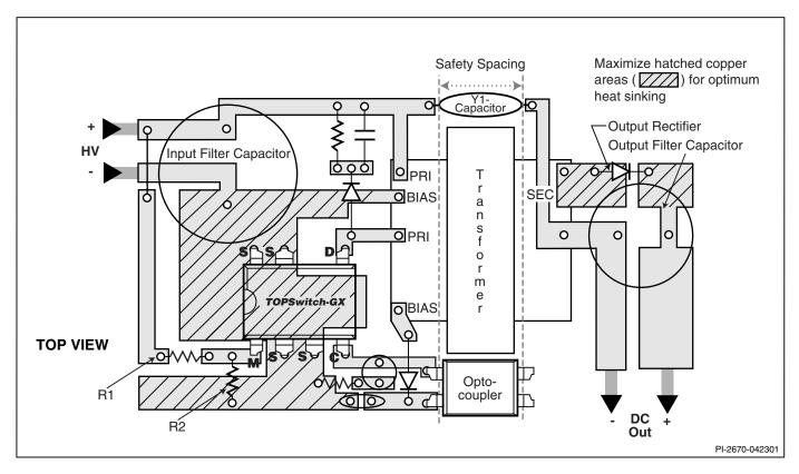
Figure 47. Layout Considerations for TOPSwitch-GX using P or G Package.
