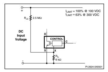
Figure 21. Current Limit Reduction with Line Voltage.
