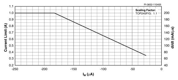
Figure 55a. Current Limit vs. MULTI-FUNCTION Pin Current (TOP245P/G only).
