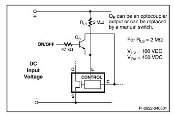
Figure 26. Active-off Remote ON/OFF with LINE-SENSE.
