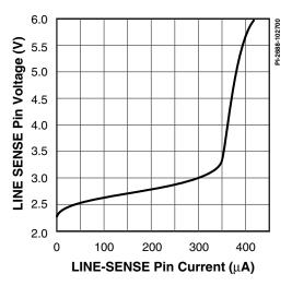
Figure 63a. LINE-SENSE Pin Voltage vs. Current.
