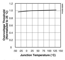
Figure 61. Overvoltage Threshold vs. Temperature.
