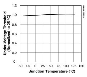
Figure 62. Under-Voltage Threshold vs. Temperature.
