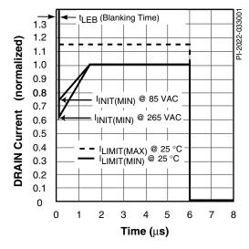
Figure 52. Drain Current Operating Envelope.
