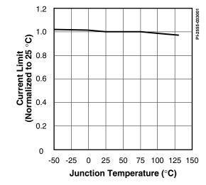
Figure 59. Internal Current Limit vs. Temperature.
