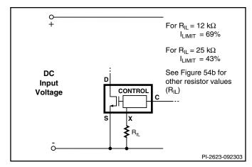
Figure 20. Externally Set Current Limit.
