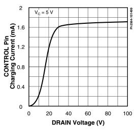
Figure 68. I<sub>c</sub> vs. DRAIN Voltage.
