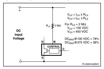
Figure 5. P/G Package Line Sense.
