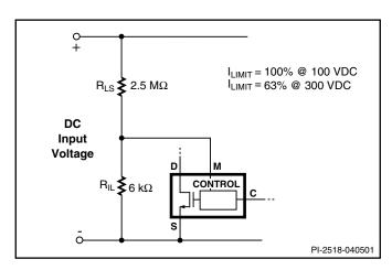
Figure 35. Current Limit Reduction with Line Voltage (Not Normally Required-See M Pin Operation Description).
