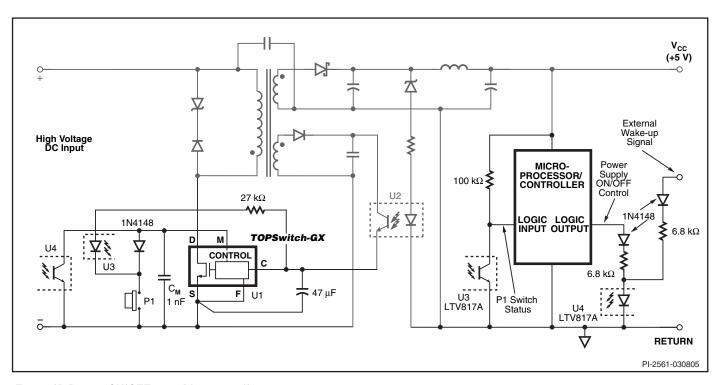
Figure 45. Remote ON/OFF using Microcontroller.
