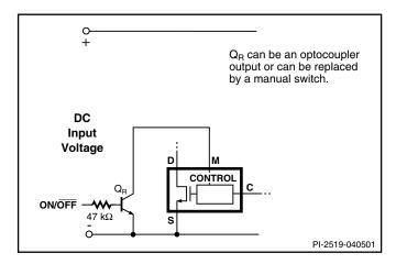
Figure 36. Active-on (Fail Safe) Remote ON/OFF.
