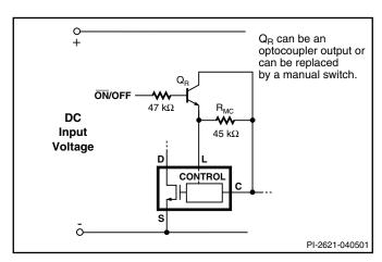
Figure 23. Active-off Remote ON/OFF. Maximum Duty Cycle Reduced.
