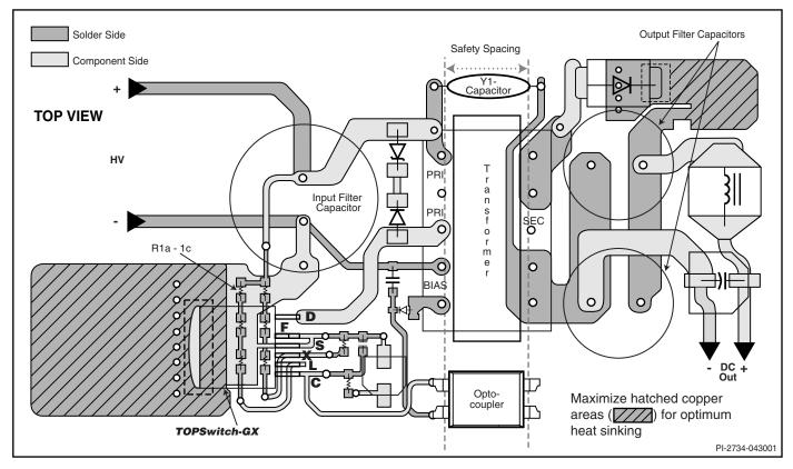
Figure 49. Layout Considerations for TOPSwitch-GX using R Package.
