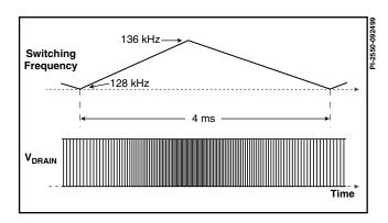
Figure 9. Switching Frequency Jitter (Idealized  $V_{DRAIN}$  Waveforms).
