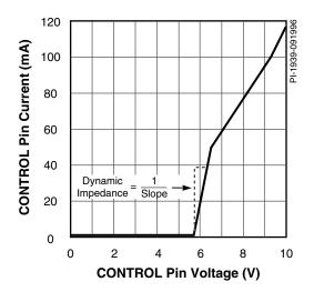
Figure 51. CONTROL Pin I-V Characteristic.
