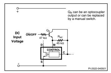
Figure 37. Active-off Remote ON/OFF. Maximum Duty Cycle Reduced.
