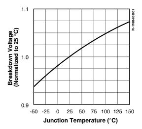
Figure 57. Breakdown Voltage vs. Temperature.
