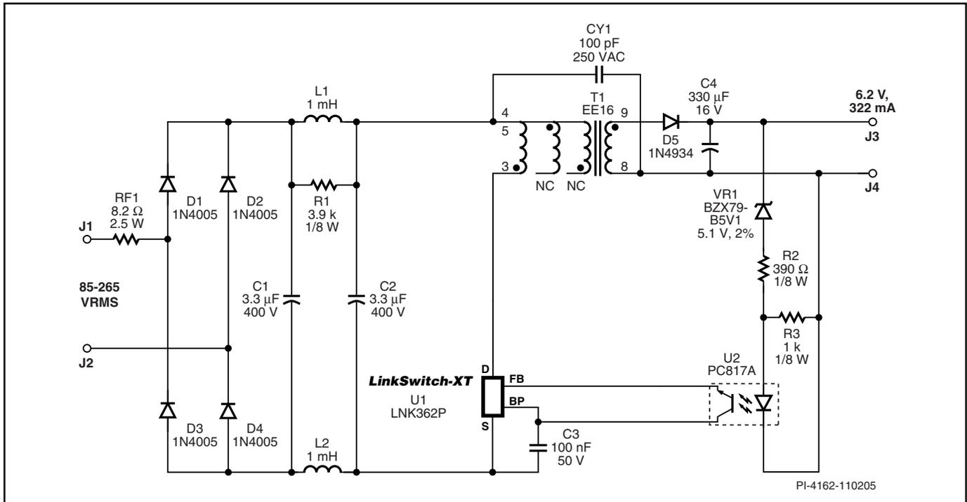
Figure 5. 2 W Universal Input CV Adapter Using LNK362.
