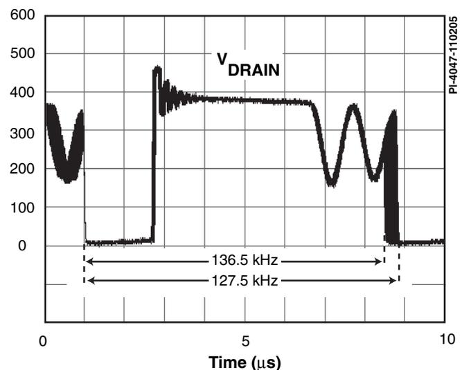
Figure 4. Frequency Jitter.
