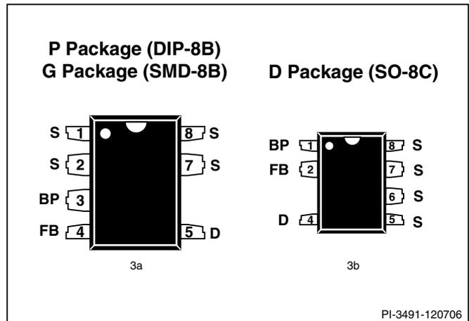
Figure 3. Pin Configuration.
