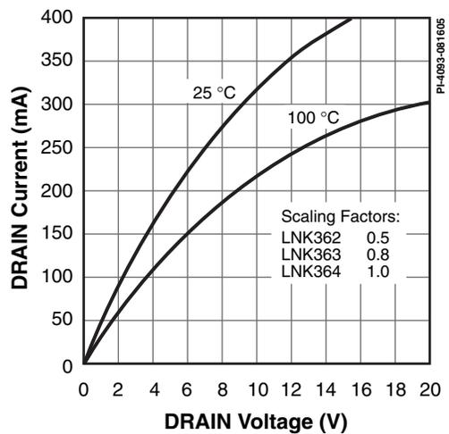
Figure 16. Output Characteristics.
