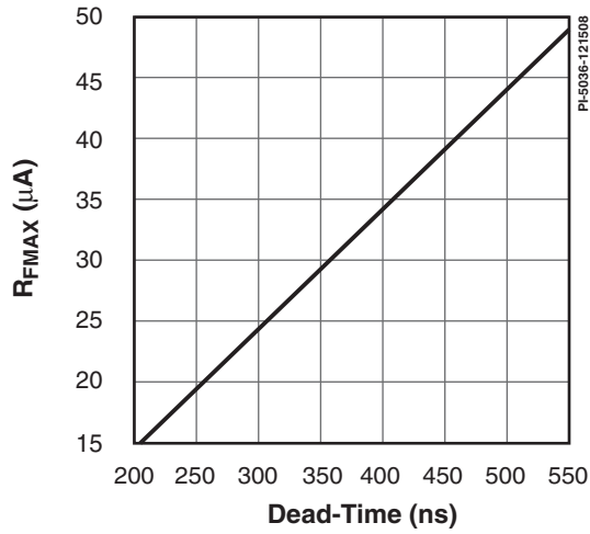
Figure 14. FMAX Pin Pull-up Resistor to VREF Pin vs. Dead-time Requirement.
