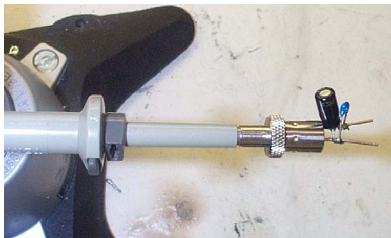
Figure 16 – Oscilloscope Probe with Probe Master 5125BA BNC Adapter (Modified with Wires for Probe Ground for Ripple measurement and Two Parallel Decoupling Capacitors Added).
