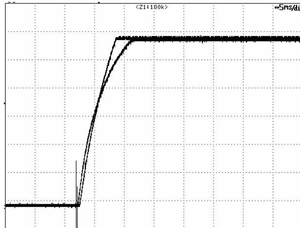
Figure 17 – Start-Up Profile, 230 VAC. Fast trace is no-load rise time Slower trace is maximum load (12 Ω) 2 V, 5 ms / div.
