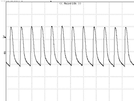
Figure 32 – Ripple, 85 VAC, Full Load, 20 mV, 20 \mu s / div.
