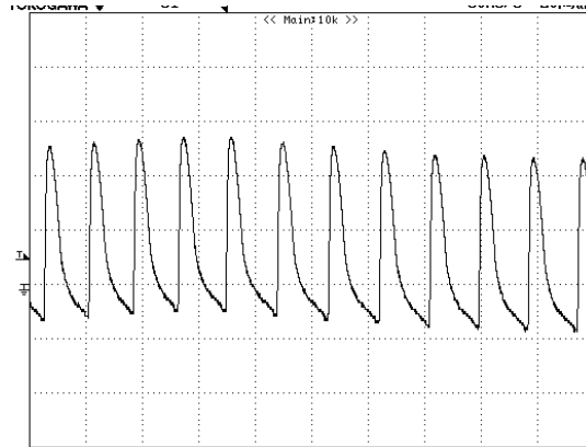
Figure 36 – Ripple, 265 VAC, Full Load, 20 mV, 20 \mu s / div.
